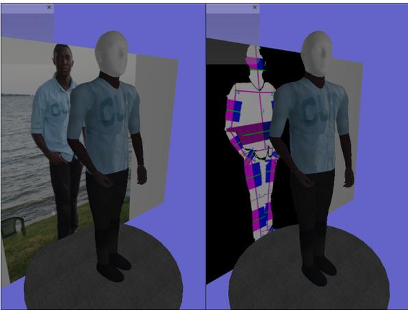
**Figure 12:** Left: the original image and the generated VH. Right: the processed silhouette and the VH.
