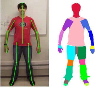
Figure 5: Illustration of the final segmentation result.
