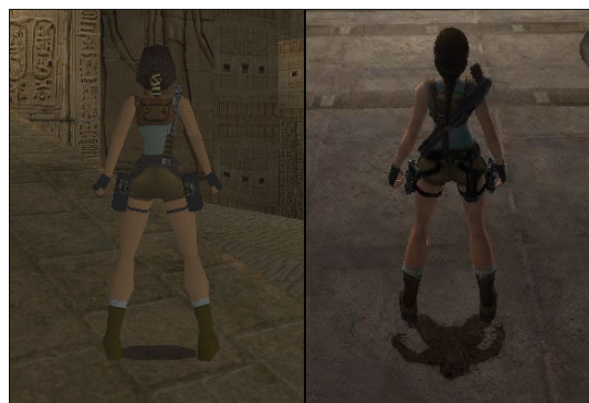
Figure 4.9 – Illustration of two types of shadowing technique present in Tomb Raider 4 game series: the simple circular shadow plane (left) and a stencil buffer technique (right).
