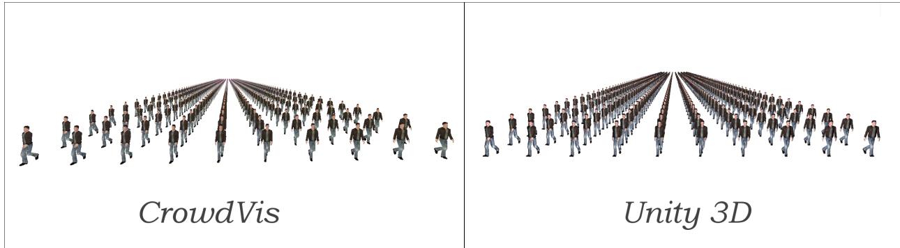
Figure 5.8 – Illustration for evaluating two different renderings, both containing 1000 agents inside the camera's frustum. On the left is illustrated the scene rendered in CrowdVis , where VHs are rendered using LOD techniques. On the right is the same scene programmed in Unity 3D , using their default rendering technique.
