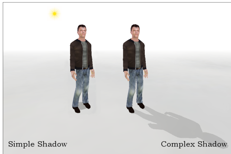
Figure 4.10 – Illustration of both shadows techniques present in CrowdVis : simple shadowing (left) and complex shadowing (right).
