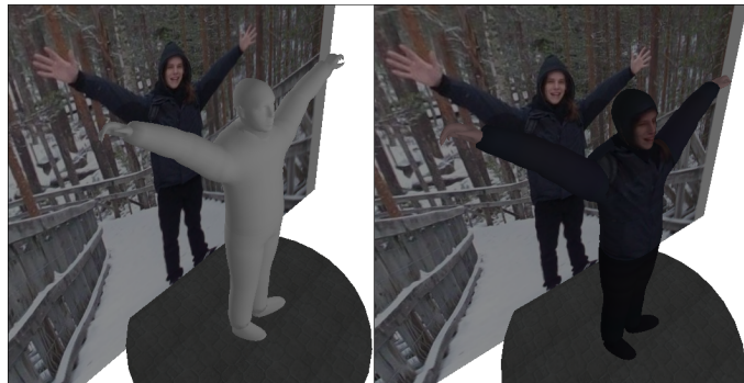
Figure 3.15 – Illustration of the template model without (left) and with (right) texture, where the color information increases the realism of the VH.
